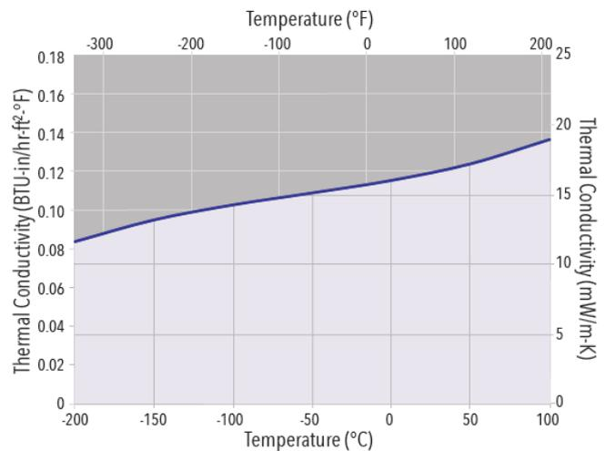
\* Thermal conductivity measured at a compressive load of 2 psi
